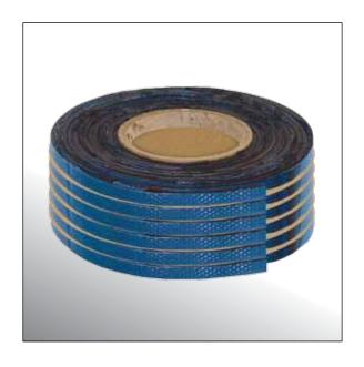
Belt Noodle Gum is an uncured rubber for hot vulcanized belt splicing. It is designed for use as a noodle rubber for steel cord belt splicing or finger splicing of fabric belts. The material is designed to bond to cured inter-core in all standard grade steel cord conveyor belts, as well as fabric belt cured skim rubber and general bond improvement material for general grade fabric conveyor belts.
