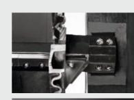
The belt consists of two PHOENOCORD belt stripes which are connected by strong rubber covered cross traverses. The material is carried by fabric reinforced rubber buckets, which are mounted to the cross traverses. All three components are connected threaded joints which allow quick and easy installation.
