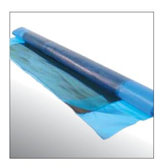
Skimmed Breaker Fabric is a Leno Weave RFL treated fabric skimmed with uncured rubber for hot vulcanized belt splicing reinforcement. It is designed for use in step splicing and finger splicing of standard grade fabric belts
