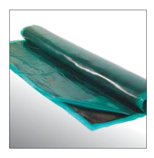
Steel Cord Belt Cover Stock is an uncured rubber for hot vulcanized belt splicing. It is designed for use as a cover rubber replacement material in splicing steel cord and fabric conveyor belts. The material is designed to bond to cured cover rubber in all standard grades of steel cord and fabric conveyor belts.
